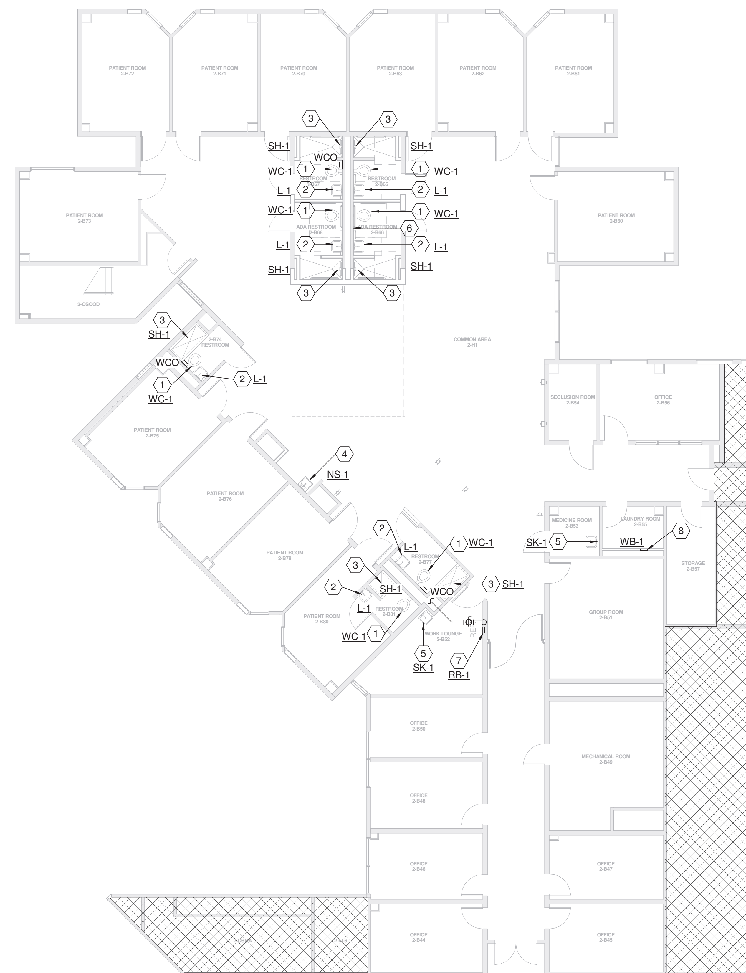
PLUMBING RENOVATION SECOND FLOOR AREA B 1/8" = 1'-0"
