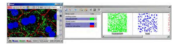
Now, the green layer is thresholded to select all of the green objects in the image. That layer is also now available in the **Binary Layers** menu. All binary layers can be selected, and their overlays seen in the image (selection was made by CTRL+clicking on the layer names, or the thumbnails)
