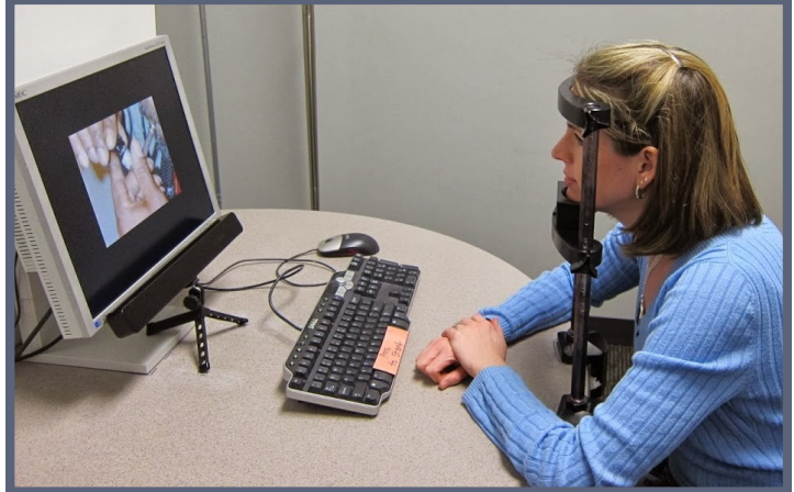
As the participant views each image, saccade eye movements are measured through an infrared eye-tracker located below the monitor.
