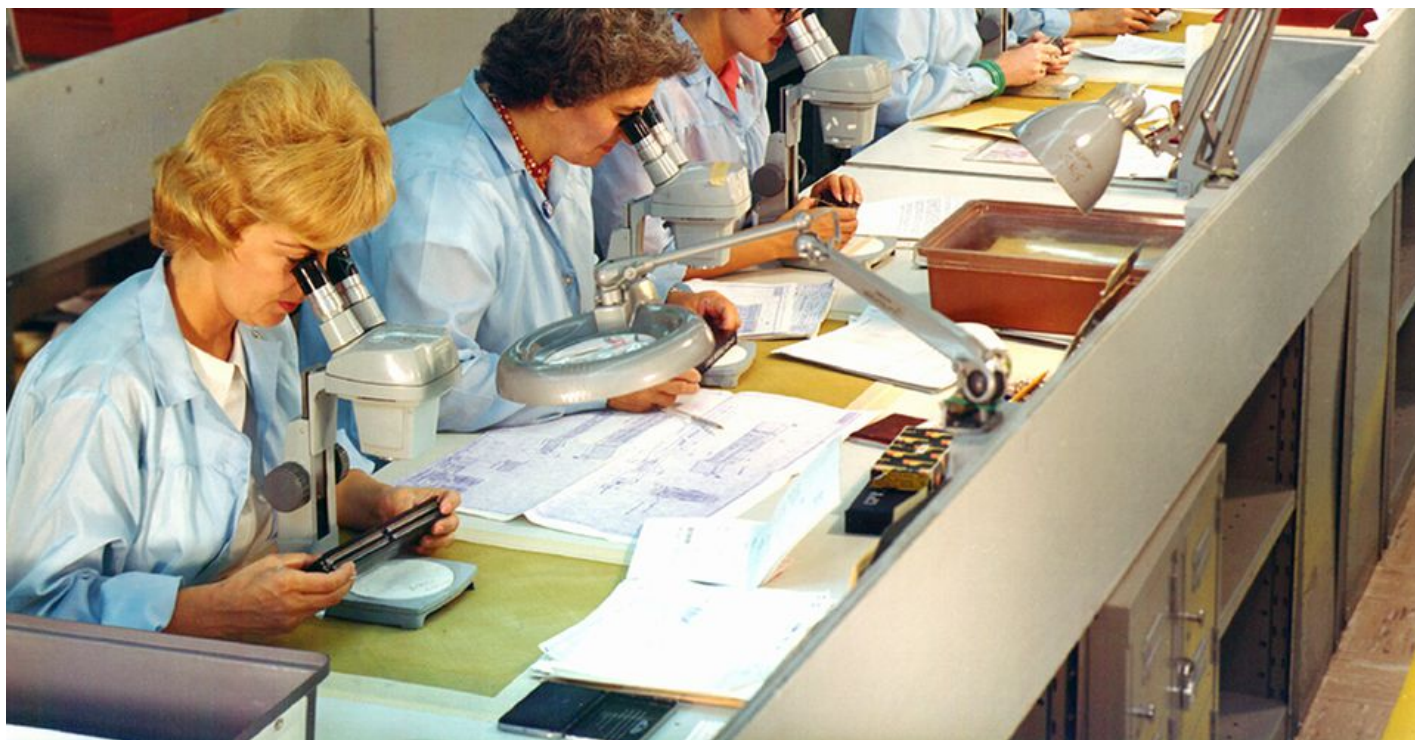
Raytheon workers stitched copper wire into the memory circuits of the Apollo spacecraft computer. (RAYTHEON CO.)
